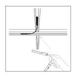
ELECTRICAL CONNECTION Every T-Connector is enclosed with one, every X connector with two flexible cross adapters. An electrical connection of the pieces can be established with these components with ease.
