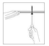
TRACK MOUNTING The track is conceived to be easily cut on site, and directly screwed to the ceiling for a tailor-made result in each in-
