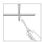
CROSSINGS Complex connection pieces belong to the past with MINIMAL TRACK. The linear elements can be used to create crossings in the easiest way. Even after the installation, adaptions can be made with minimal effort.
