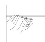
INSERTS Place and remove any insert wherever you want by simply pulling it out and snapping it in without any tools needed.
